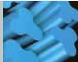
Because of the trilobal shape of the fiber soil stays on the surface which makes cleaning easier.
